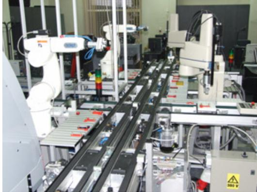
Fig. 1.7. Layout of the manufacturing cell with holonic control
